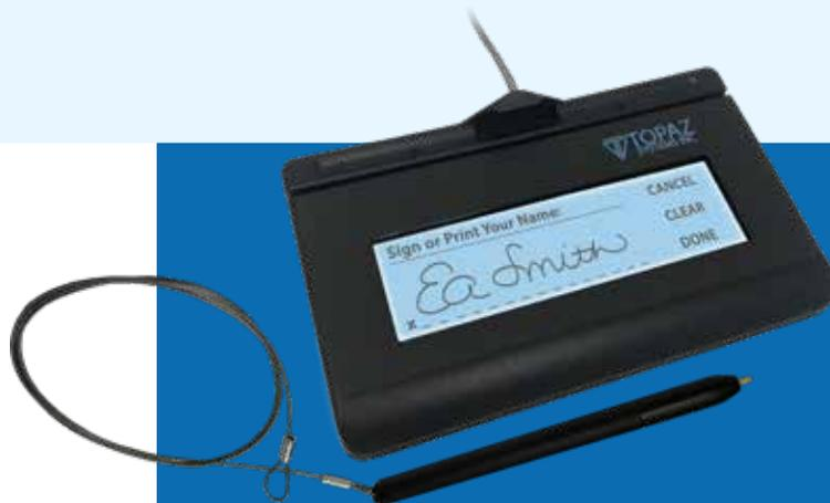
The Topaz® KioskGem™ LCD 1x5 is a small, rugged, advanced electronic signature pad with transfective LCD that displays “electronic ink” under the pen tip during signing. It is designed for public-access and kiosk-mount application. The KioskGem LCD 1x5 mounts to a surface with no exposed cables or fasteners, and the pen is connected with a high-stress tether rated at 160 lbs.
