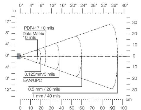
\* The reading distances for each scanner are typical distances measured from the front end of the scanner bezel in an office environment (200 lux) with extended reading range activated.
